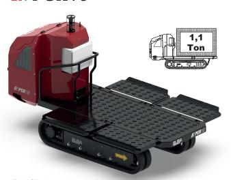
The PCR10 is a crawler vehicle without stabilisers and with a platform load capacity of 1.1T.
